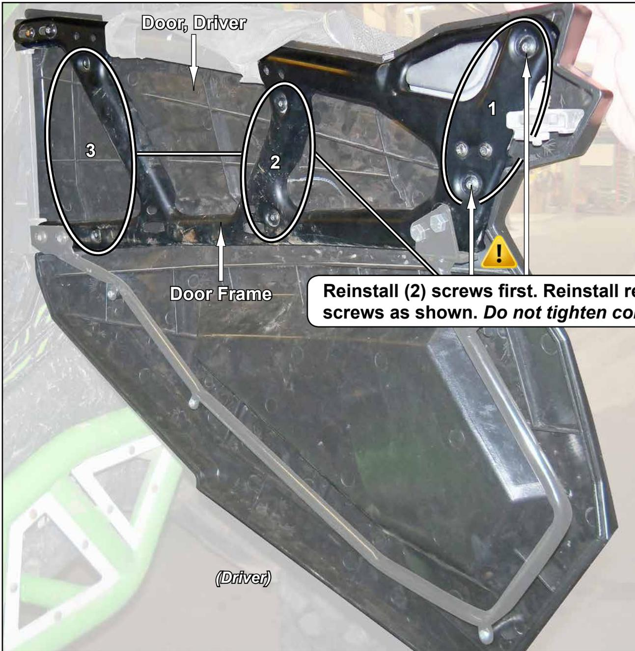
3. Secure Brace, Driver to Door, Driver with 1/4"-14 x 3/8" Lg. PHMS.
