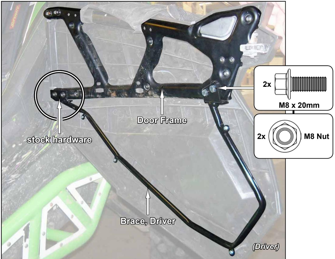
2. Install stock Door Frame to Door, Driver with stock hardware.
